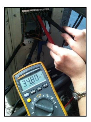
Pic 1: Use a multimeter to test the DC voltage between 2(old: L2) port and 3 port of outdoor unit. The red pin of multimeter connects with 2 (old: L2) port while the black pin is for 3 port.
