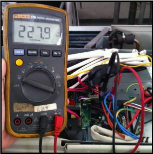
2 Turn off the power, use a digital tester to measure the resistance. The value should be 1.8~2.5  $K\Omega$ .
