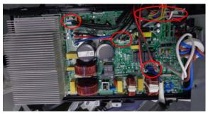
8) Disconnect the grounding wire (yellow - green) after removing the big handle and the right-rear panel.
