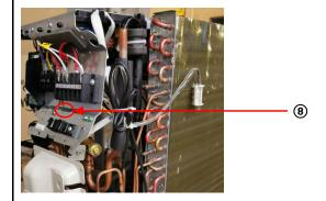
9) Remove the PCB board.
