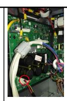
3) Disconnect following 8 pieces of connection wires and connectors between IPM and other parts.
